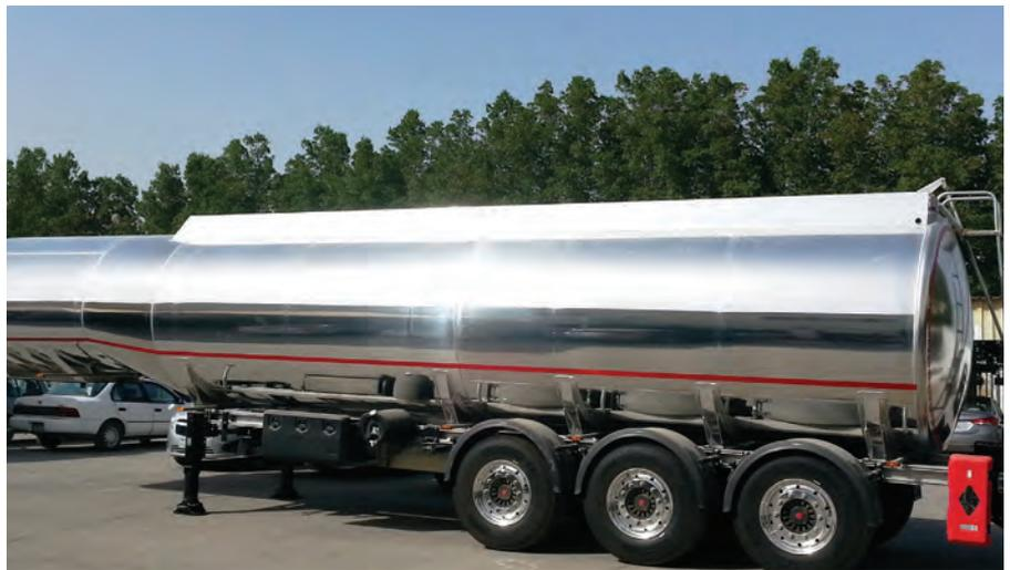
equipped with BPW or SAF axles, bottom loading system, air brake system, ABS/EBS system, LED electrical system, Michelin tires and aluminum rims.
